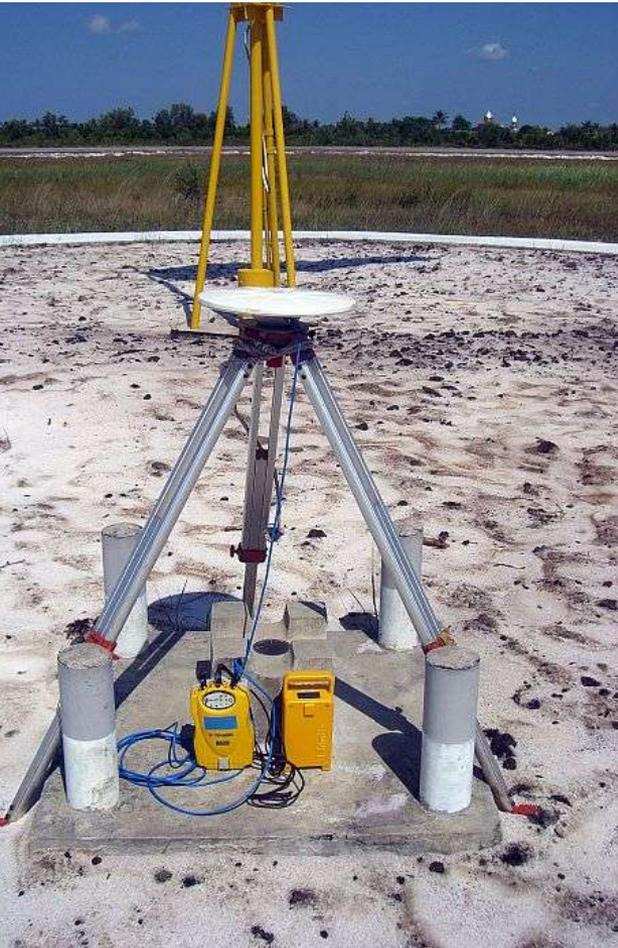
**Orthometric Height = GPS ellipsoidal Height - Geoid Height**
