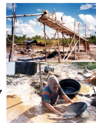
SSGM-Technology using Dulang and Mercury at Galangan taken in June 1998 near Kereng Pangli near to the main road
