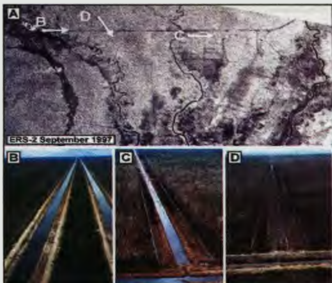
Figure 7. Irrigation channels of the 1 million ha rice project. A: Gamma map filtered ERS-image mosaic showing irrigation Channels (PPC, MPC, SC, TC) of the MRP at the Kapuas River region. (ERS images acquired 18 September 1997 and 2 September 1997.) B: Main Channel, 110 km long, C: Side channel filled with water near Kapuas river, D: Dried out side channel in the centre of the peat dome between Kahayan and Kapuas river. Burnt scars are visible along the channels.
