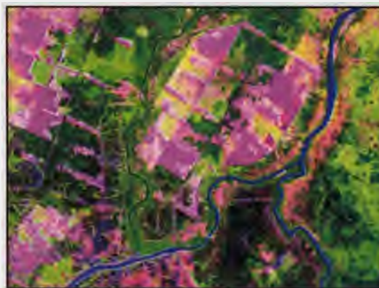
Figure 10. LANDSAT-image (RGB = 543) taken from the MRP in Central Kalimantan at Dadahup on 29 May 1997 (30 km x 42 km). PSF is in green colour, clear-cut, see red colours and many new channels were dug. This image shows the situation before the huge fires in autumn 1997 and spring 1998. Now there are more than 4,000 km of channels in the MRP which has many problems in hydrology of draining instead of irrigating the land and in big peat layers which are not suitable for rice cultivation.
