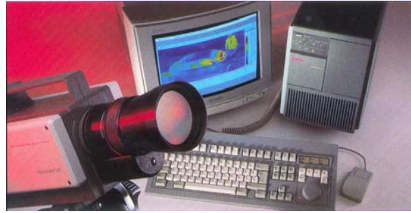
Fig. 5: Sensorhead, processor and special keyboard of the AGEMA-camera.
