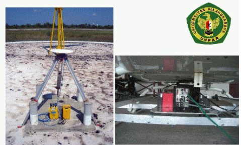
Photo from DGPS-station (left) and ALS-, INS- and RGB-camera equipment under the helicopter
